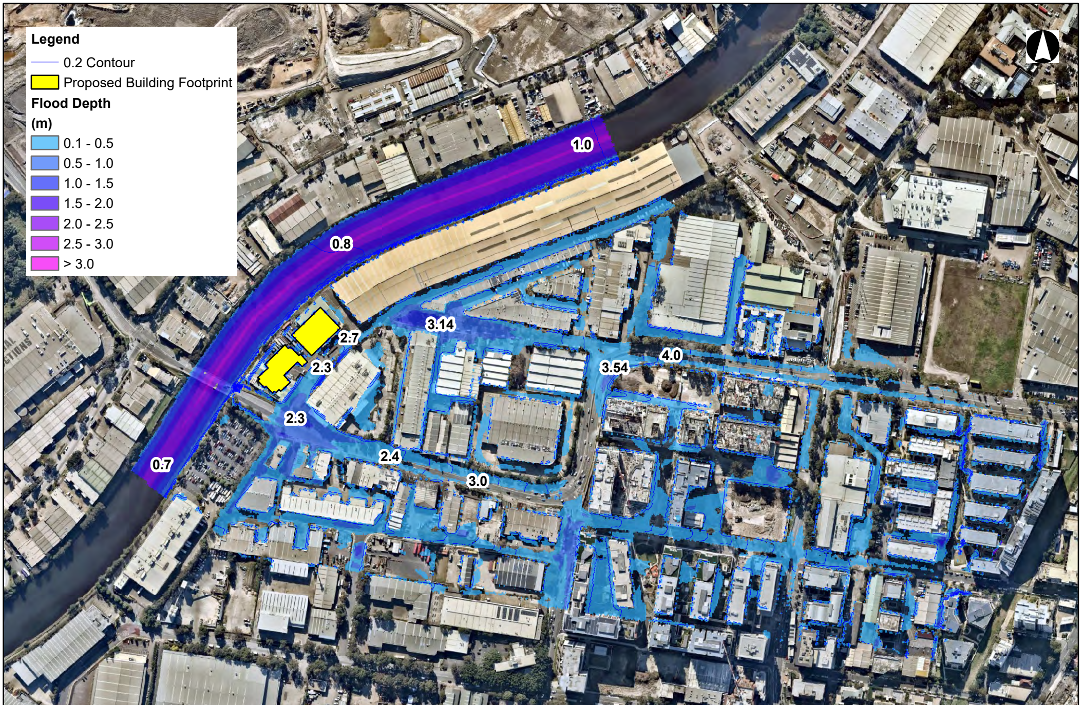
Figure F8 1%AEP, 0.7 m AHD TWL, Proposed Conditions Flood Depths
