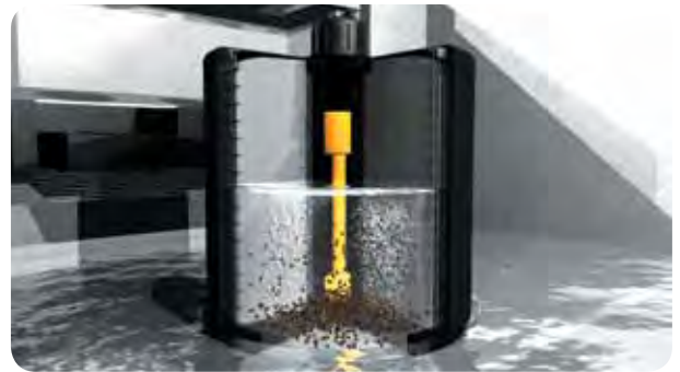
Enhanced Filtration through StormFilter
