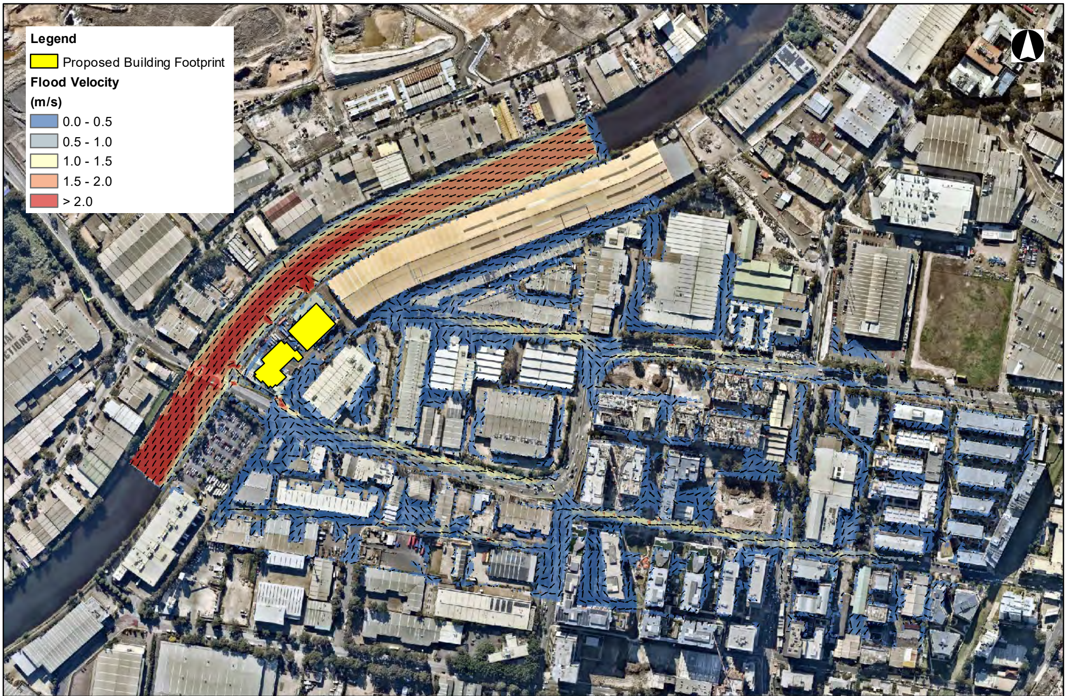
Figure F11 1% AEP, 0.7 m AHD TWL, Proposed Conditions Flood Velocity
