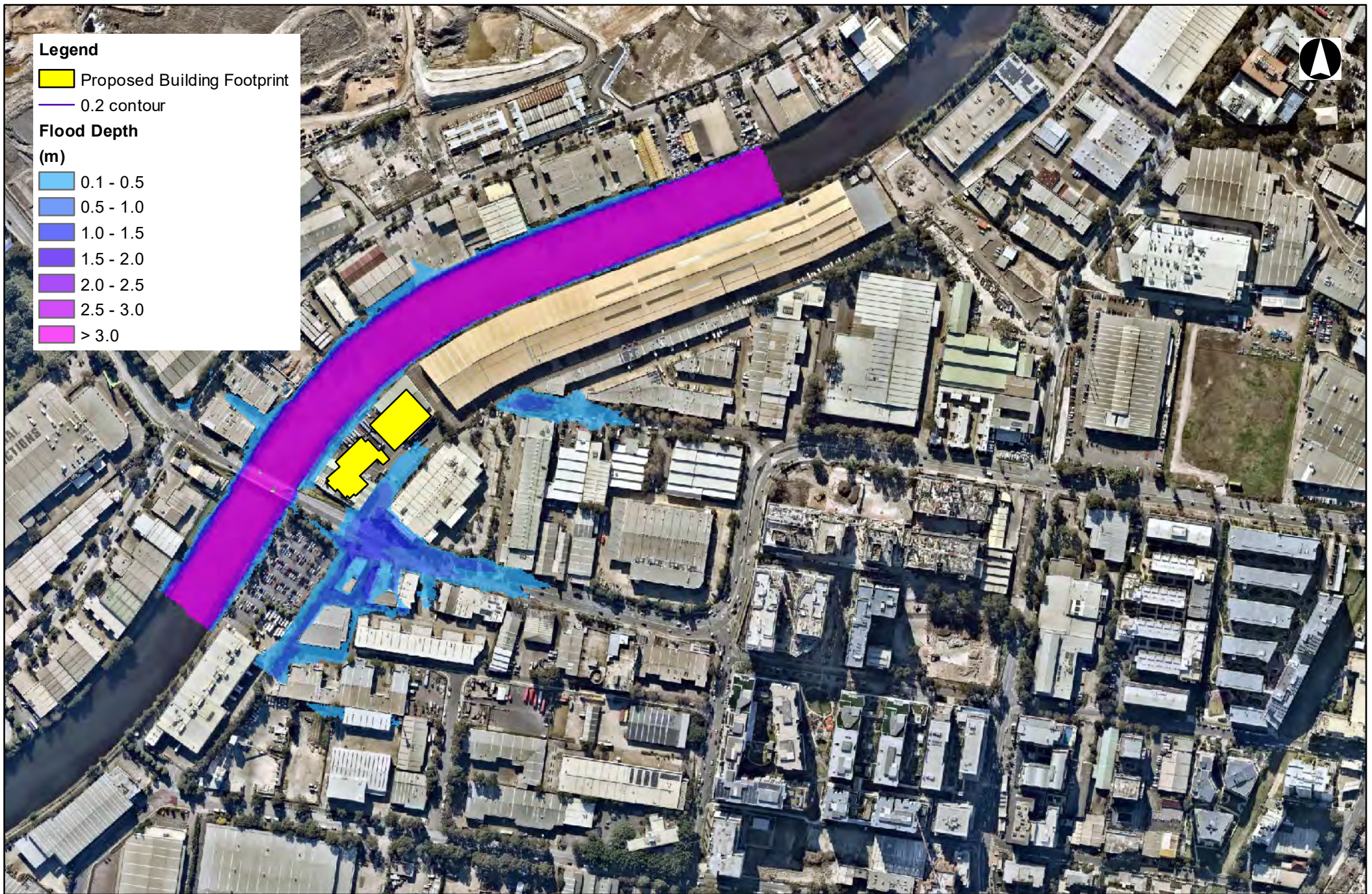
Figure F9 No Rainfall, 2.5 m AHD TWL, Proposed Conditions Flood Depths
