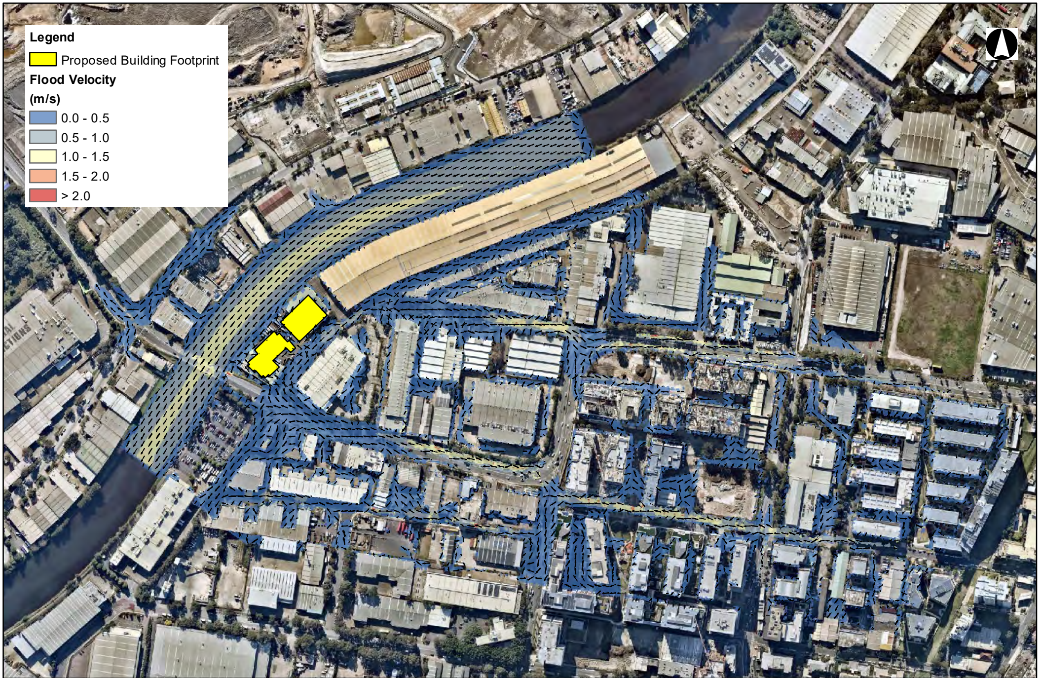
Figure F10 1% AEP, 2.5 m AHD TWL, Proposed Conditions Flood Velocity
