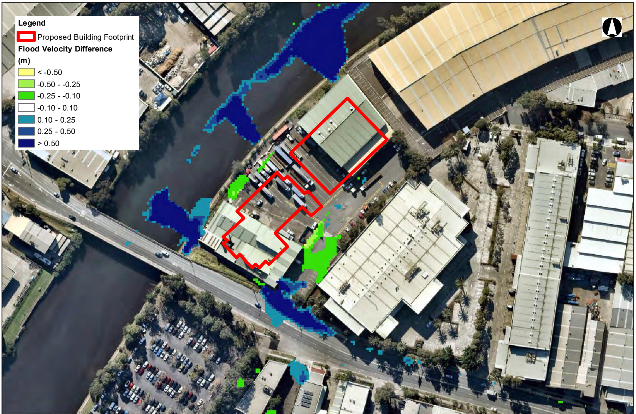
Figure F18 No Rainfall, 2.5 m AHD TWL, Proposed Conditions Flood Velocity Difference
