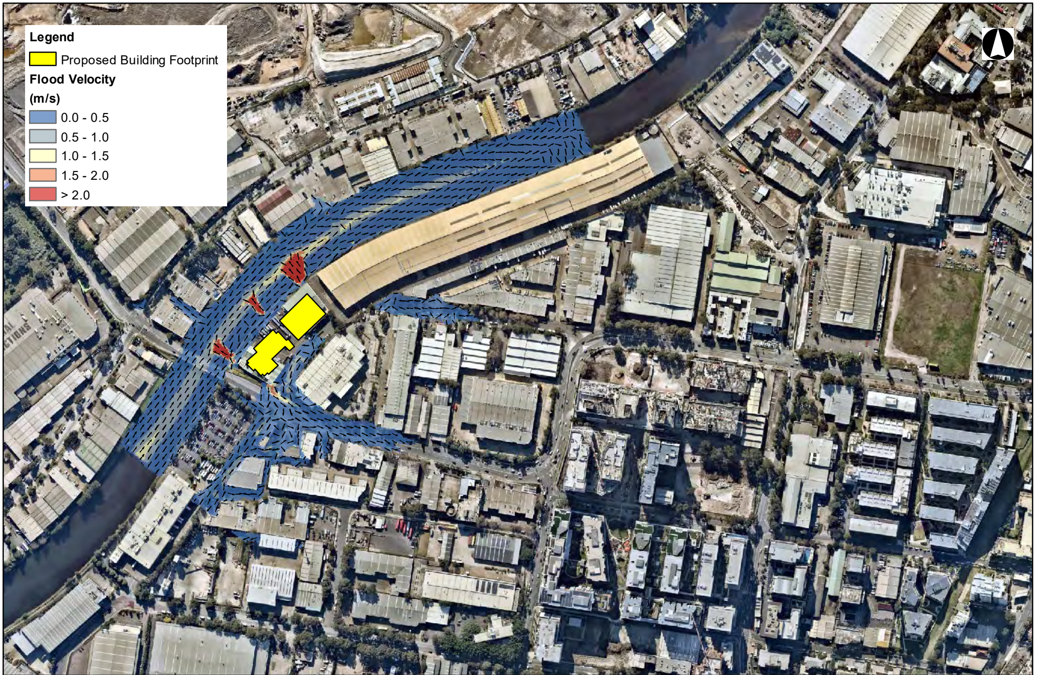
Figure F12 No Rainfall, 2.5 m AHD TWL, Proposed Conditions Flood Velocity
