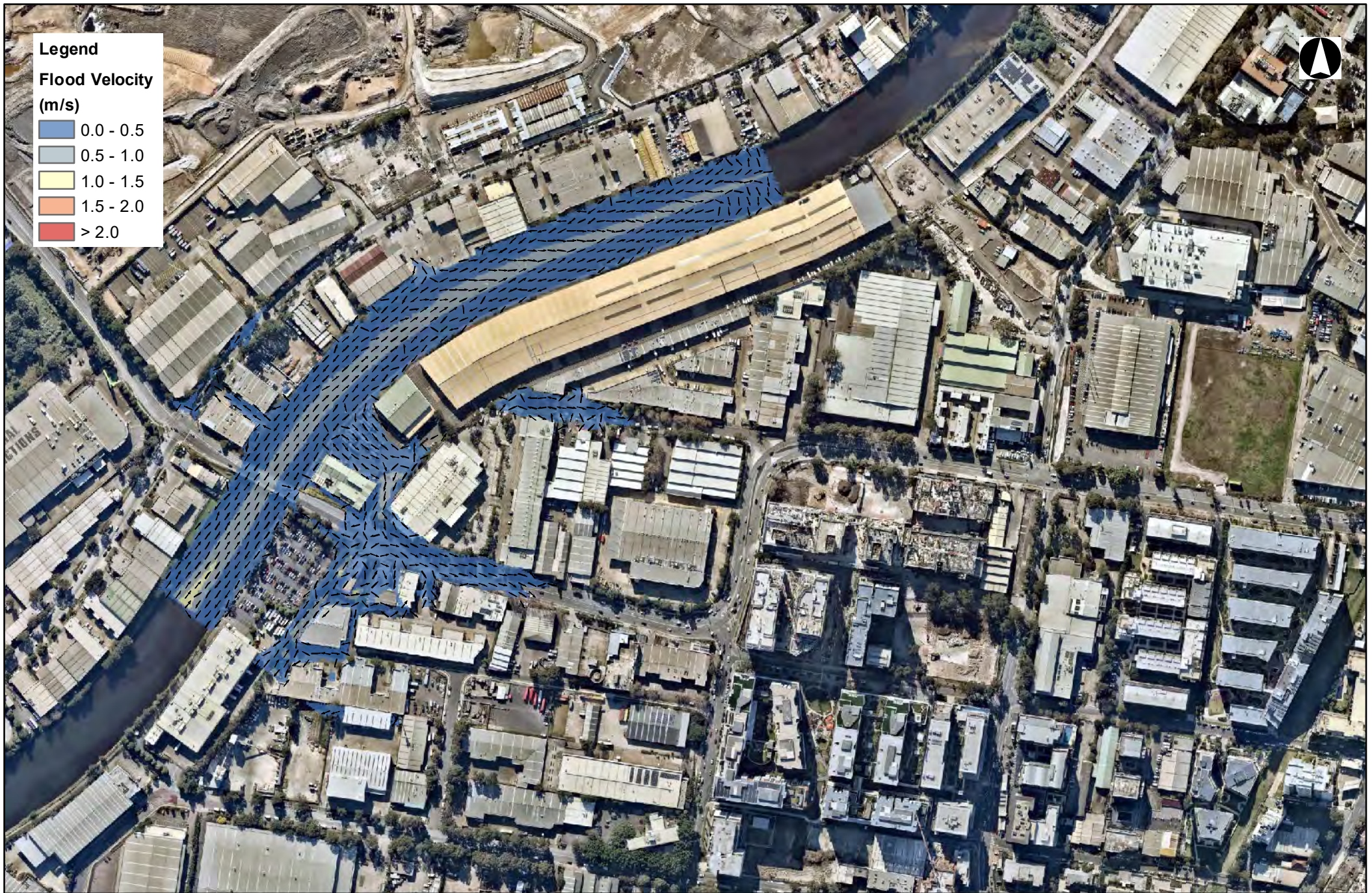
Figure F6 No Rainfall, 2.5 m AHD TWL, Existing Conditions Flood Velocity
