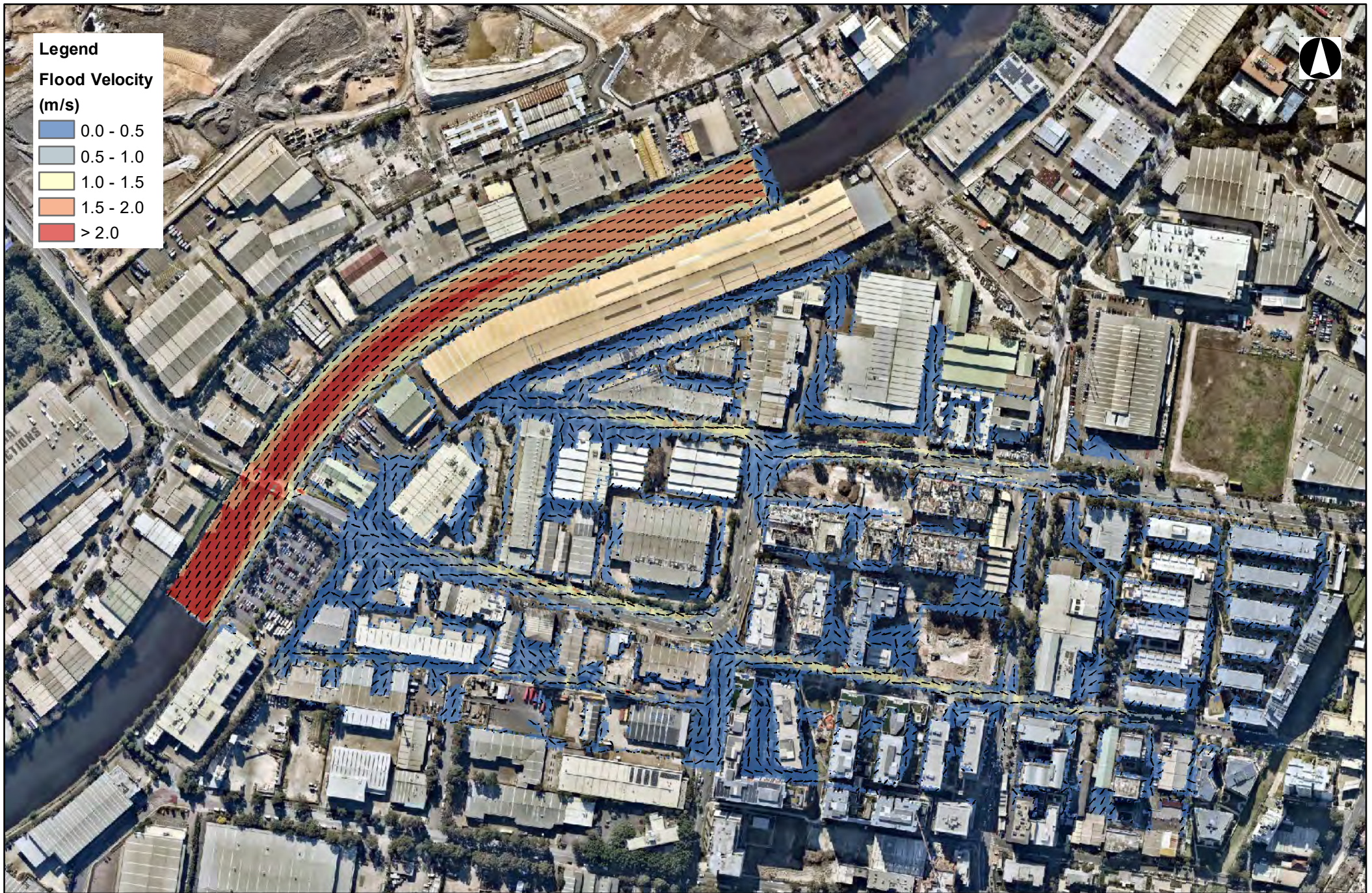
Figure F5 1% AEP, 0.7 m AHD TWL, Existing Conditions Flood Velocity
