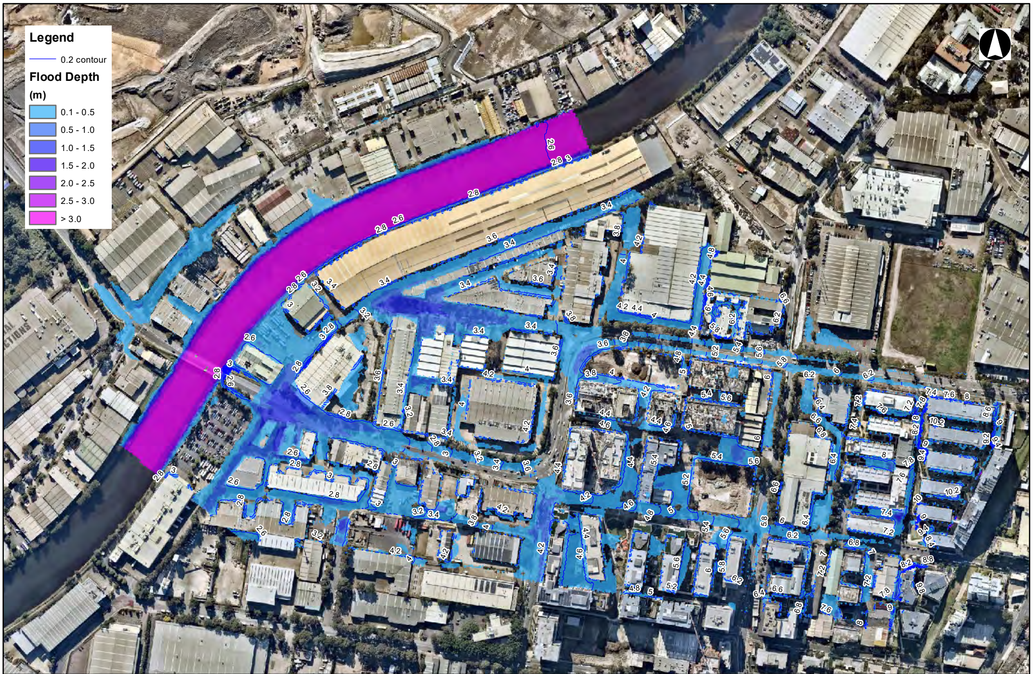
Figure F1 1% AEP, 2.5 m AHD TWL, Existing Conditions Flood Depths
