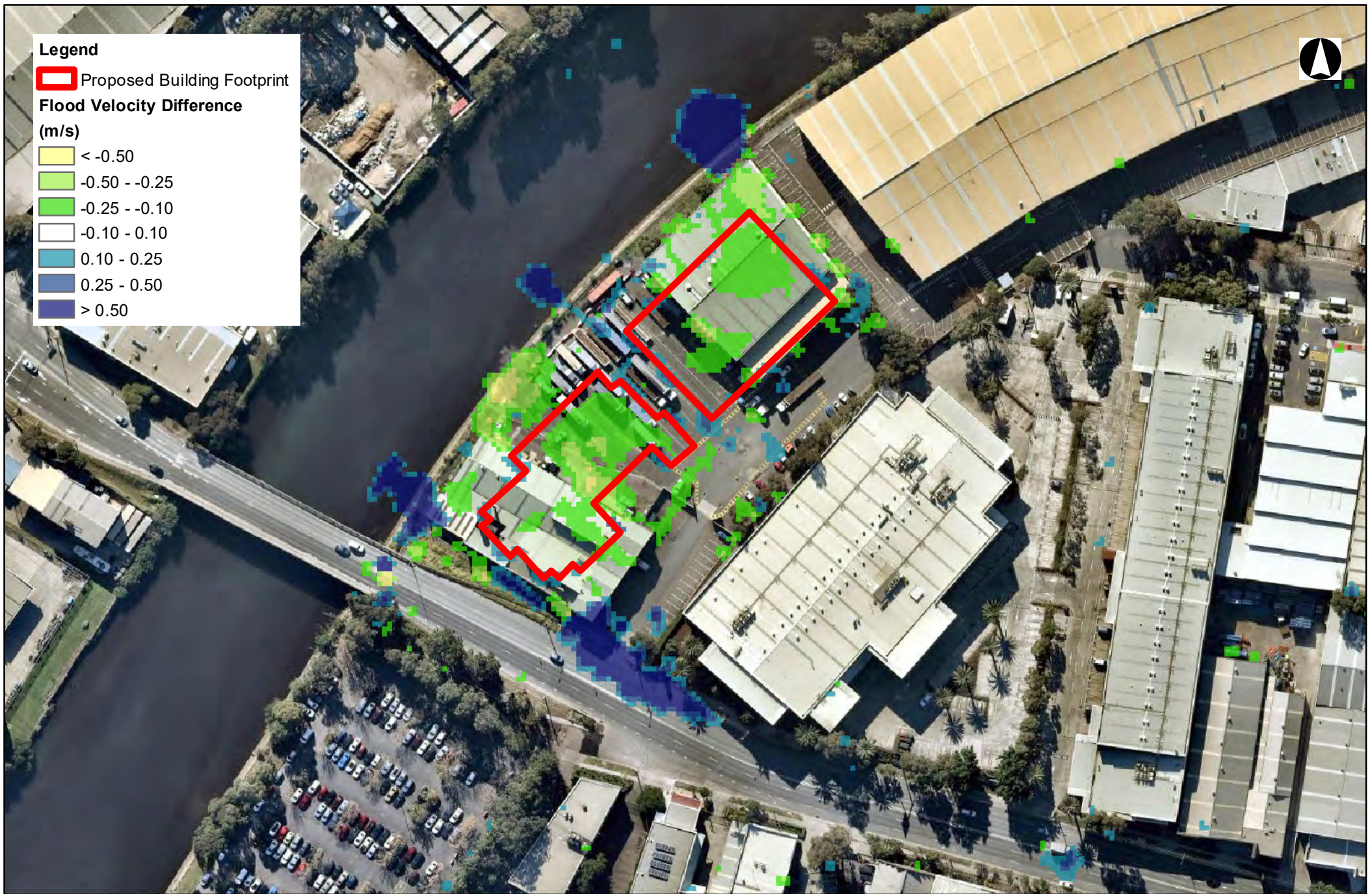
Figure F16 1%AEP, 0.7 m AHD TWL, Proposed Conditions Flood Velocity Difference
