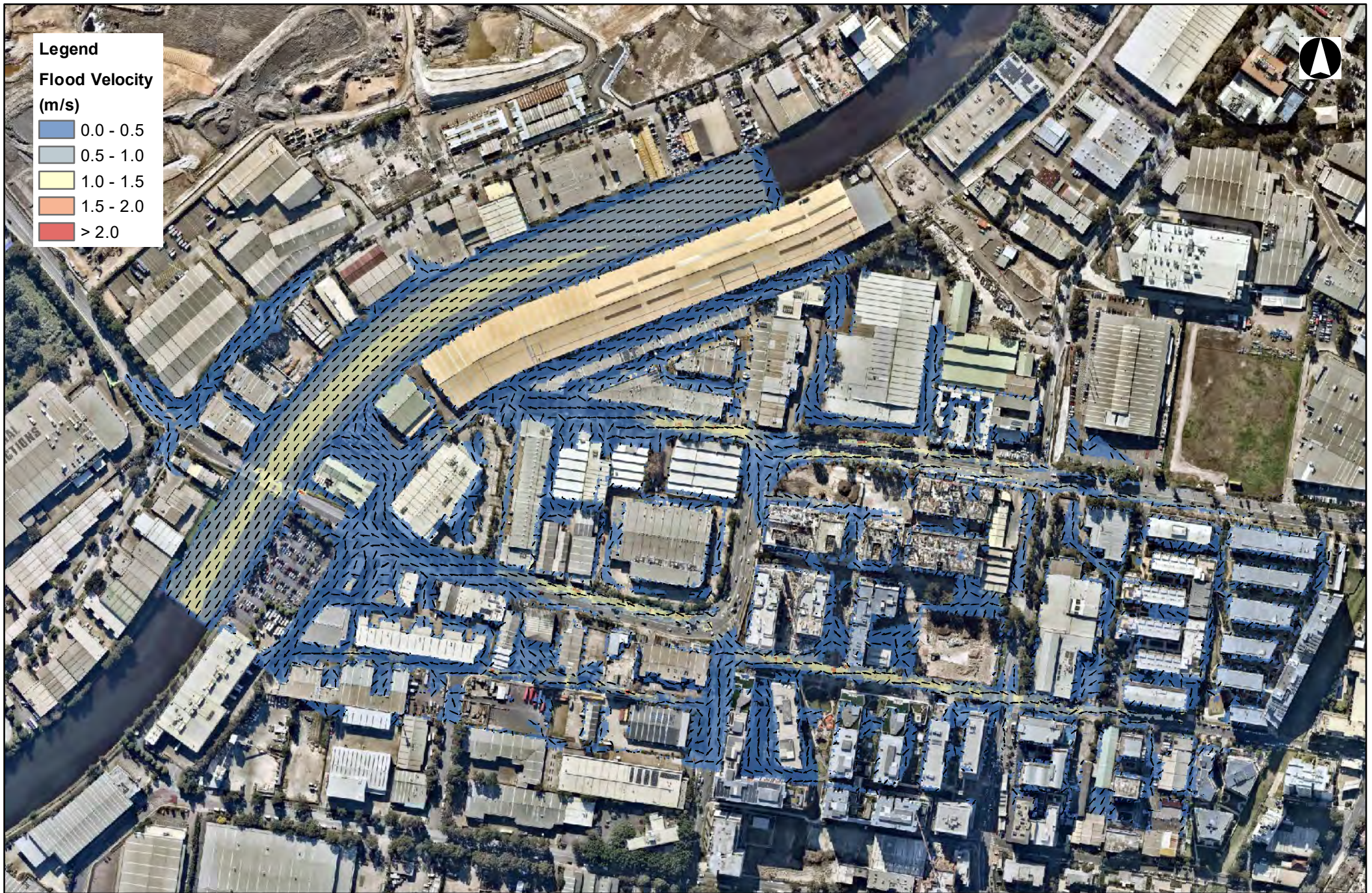
Figure F4 1% AEP, 2.5 m AHD TWL, Existing Conditions Flood Velocity
