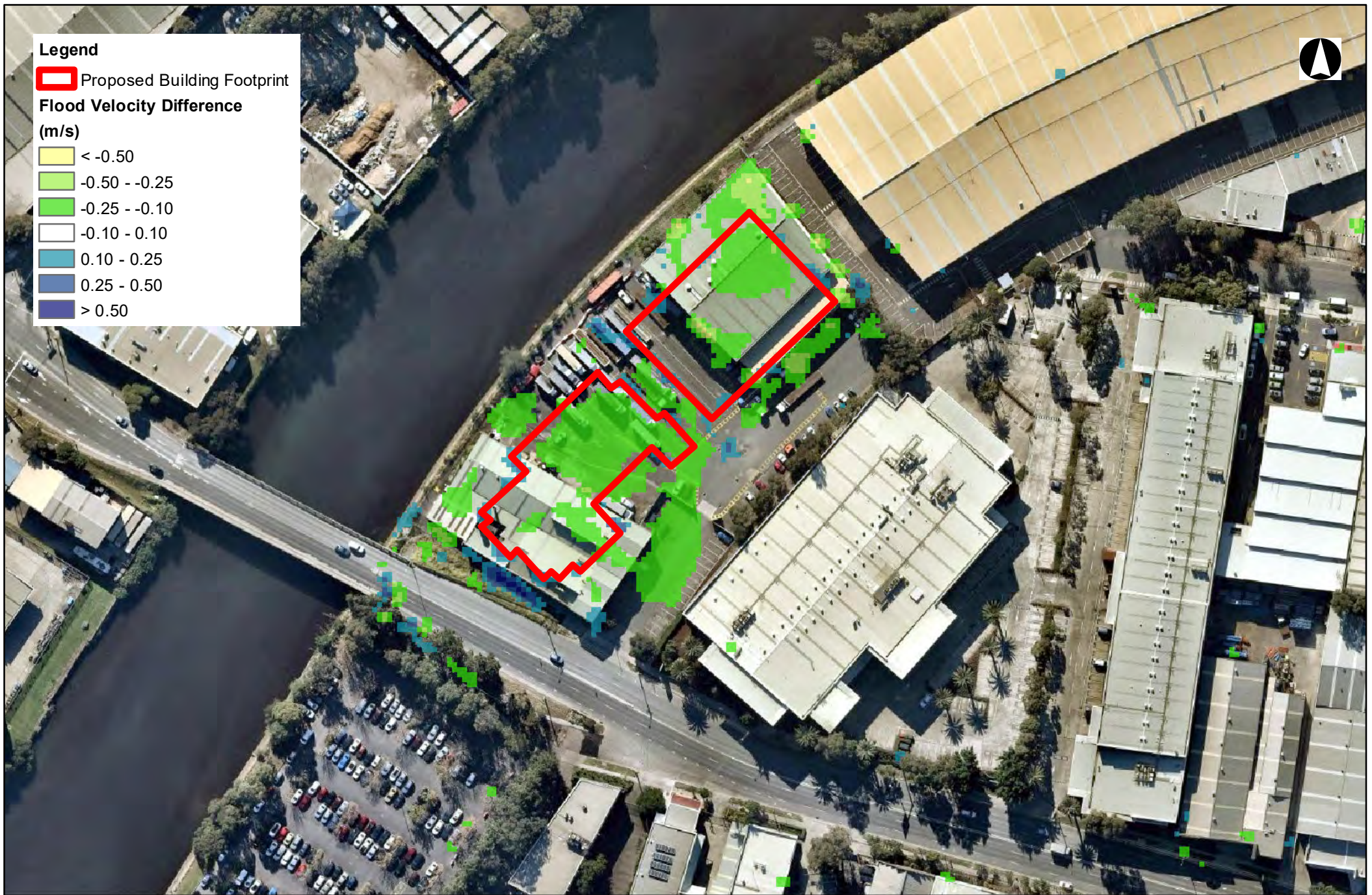
Figure F14 1%AEP, 2.5 m AHD TWL, Proposed Conditions Flood Velocity Difference
